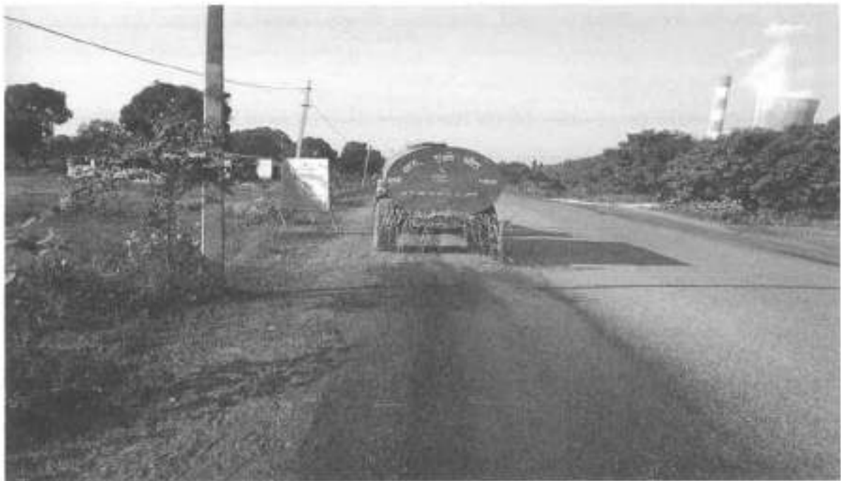
Photo 16: Regular water sprinkling is carried out on the main roads near the plant-affected villages. Additionally, the main roads are cleaned through routine brooming to maintain cleanliness and improve the surrounding environment.
